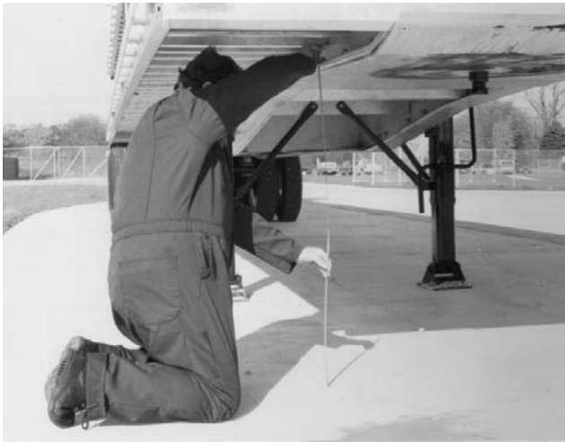
Figure 12. Measuring the actual kingpin height
