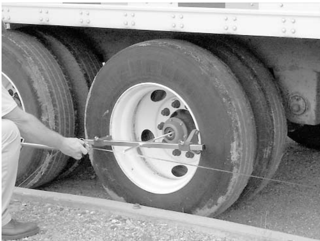
Figure 19. Measuring the "A" and "B" distances
